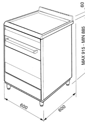
NB: Height with plinth installed is fixed at 900mm
