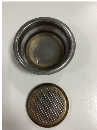
Sediments can be seen in this opened filter.
